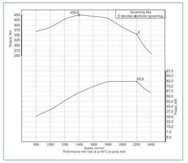
Rating Conditions for Diesel Engines – up to 7.1 litres are based on ISO/TR14396, inlet air standard conditions with a total barometric pressure of 100 kPa (29.5 in. Hg), with a vapour pressure of 1 kPa (0.295 in Hg) and 25°C (77°F). Performance is measured using fuel to specification EPA 2D 89.330-96 with a density of 0.845-0.850 kg/L @ 15°C (59°F) and fuel inlet temperature 40°C (104°F).
