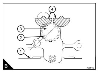
**7** Fit the two dowels to the rear face of the balancer frame. Lubricate the bushes in the rear cover of the balance frame with clean engine lubricating oil. Put the rear cover (page 82/A4) in position with the rear spigots of the balance weights in the bushes of the cover. Hit lightly the rear cover with a soft face hammer to fit the cover onto the dowels. Fit the cover setscrews and tighten them to 54 Nm (40 lbf ft) 5,5 kgf m.
