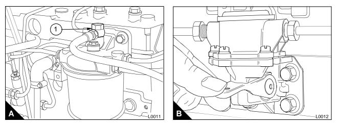
**3** Ensure that the manual stop control is in the "run" position. If an electrical stop control is used, turn the start key to the "R" position.
