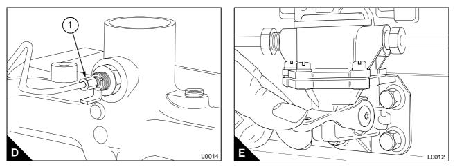
**6** Loosen the union nuts (F1) of the high-pressure pipes a half turn at two of the atomisers. Operate the starter motor until fuel free from air, comes from the pipe connections. Tighten the high pressure pipe connections to 22 Nm (16 lbf ft) 2,2 kgf m.
