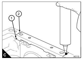
*Caution:* When the sump joint is removed, damage can occur to the seal in the grooves of the bridge piece. If the seal is damaged, apply enough sealant to completely fill the grooves.
