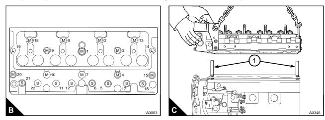
**7** Tighten the setscrews, in the correct sequence, a further part of a turn according to the length of the setscrews, see (B). Short setscrews (S) must be turned a further 150° (2.5 flats). Medium length setscrews (M) must be turned a further 180° (3 flats). Long setscrews (L) must be turned a further 210° (3.5 flats). A special tool (D) can be used for this operation.
