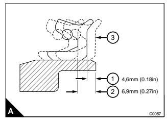
If all positions have been used it is permissible to grind the crankshaft flange, refer to the relevant Data and dimensions for the "Crankshaft" on page 18.
