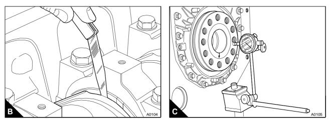
If the end-float is more than the tolerance given in the relevant Data and dimensions for the "Crankshaft" on page 18, thrust washers which are 0,019 mm (0.0075 in) oversize can be fitted.
