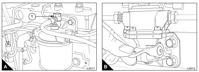
**Note:** If the drive cam of the fuel lift pump is at the point of maximum cam lift, it will not be possible to operate the priming lever. In this situation, the crankshaft must be rotated one revolution.
