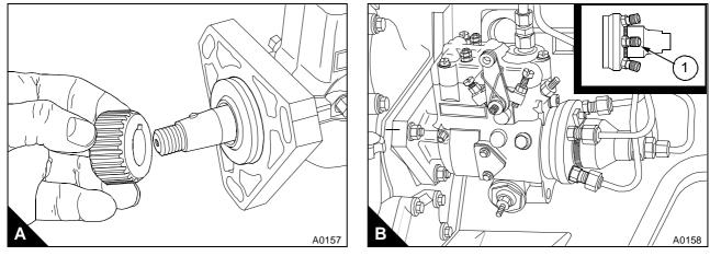
**4** Rotate the drive shaft of the fuel pump clockwise from the drive end of the pump until the pin in the shaft aligns with number 1 outlet. Loosen the screw (C3) on the timing tool MS.67B and set the timing tool to the correct pump mark angle, see "Static timing - Stanadyne fuel injection pump" on page 24. Tighten the screw.
