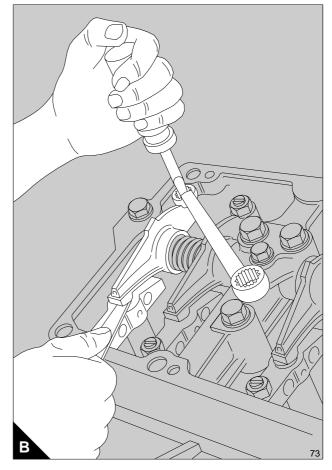
Check the tappet clearance AFTER the bridge pieces have been adjusted. When the clearance has been set correctly (B), tighten the lock nut to a torque of 40 Nm (30 lbf ft).
