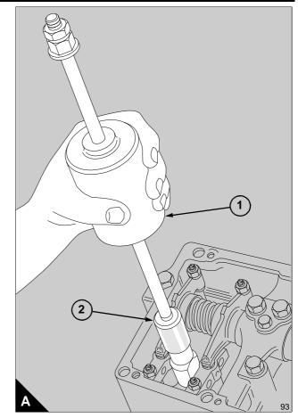
**3** Fit the assembly of the metal cup and rubber seal against the head of each connection for leak-off fuel and fit a new copper washer onto the thread. For **early engines**, insert each connection through the openings in the outer walls of the rocker boxes and fit the connection into its fuel injector, finger-tight.
