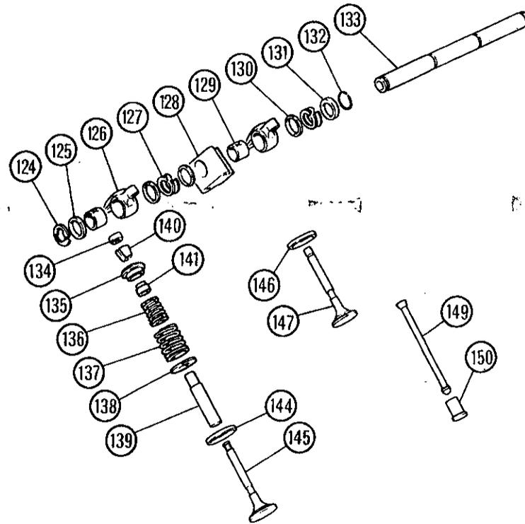
**Fig. 25** Valves and rocker assembly
