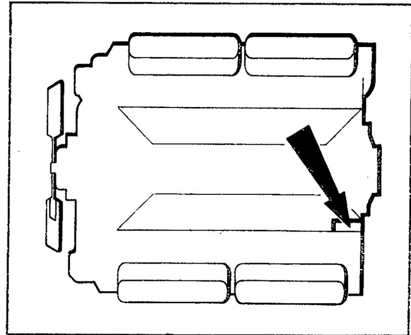
Fig. 2 Engine number position
