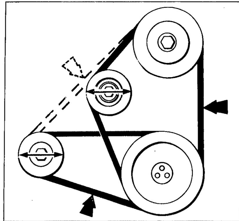
Fig. 11 Drive belt tension adjustment
