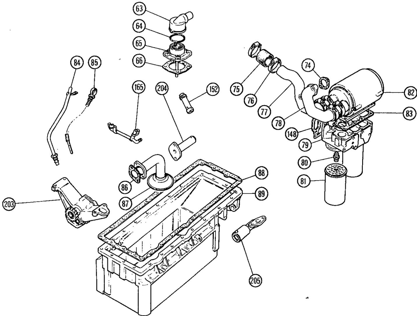
**Fig. 29** Lubrication system components
