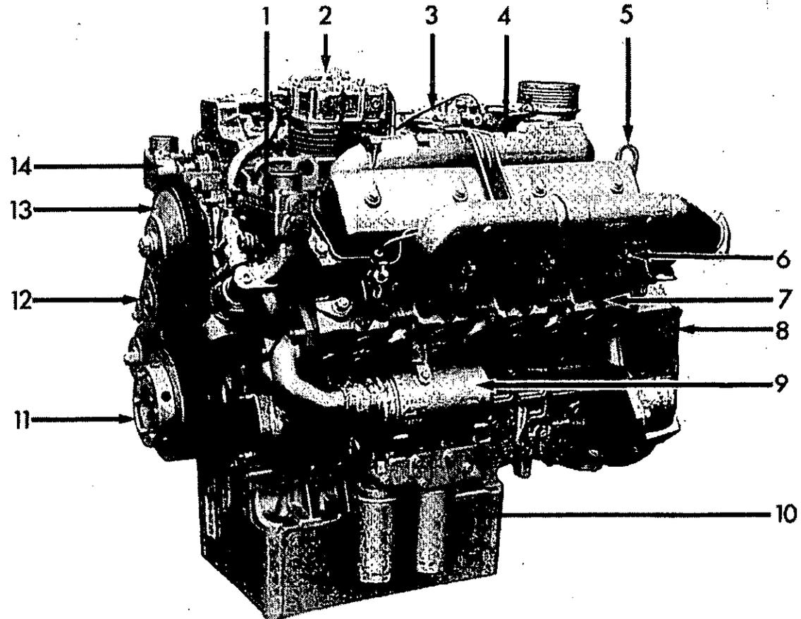
Fig. 3 Front left side of V8.640 engine.
