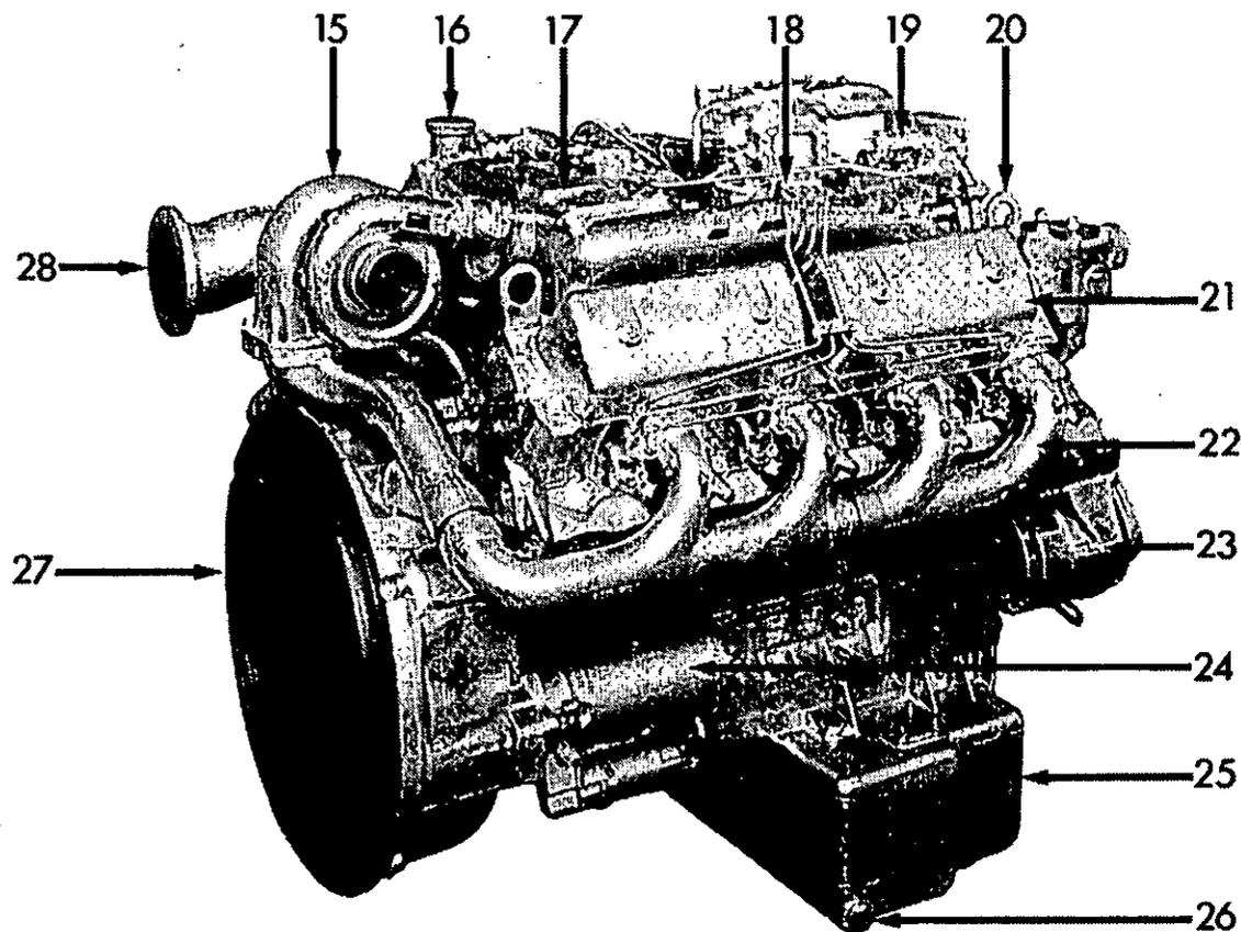
Fig. 4 Rear right side of TV8.640 engine
