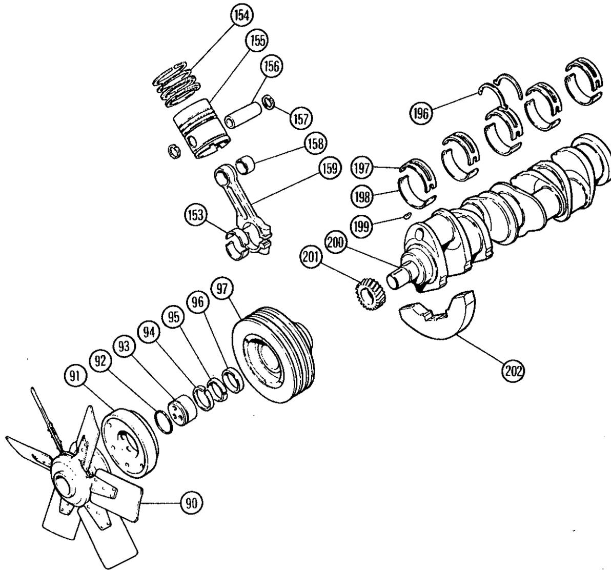
**Fig. 26** Crankshaft and piston assemblies
