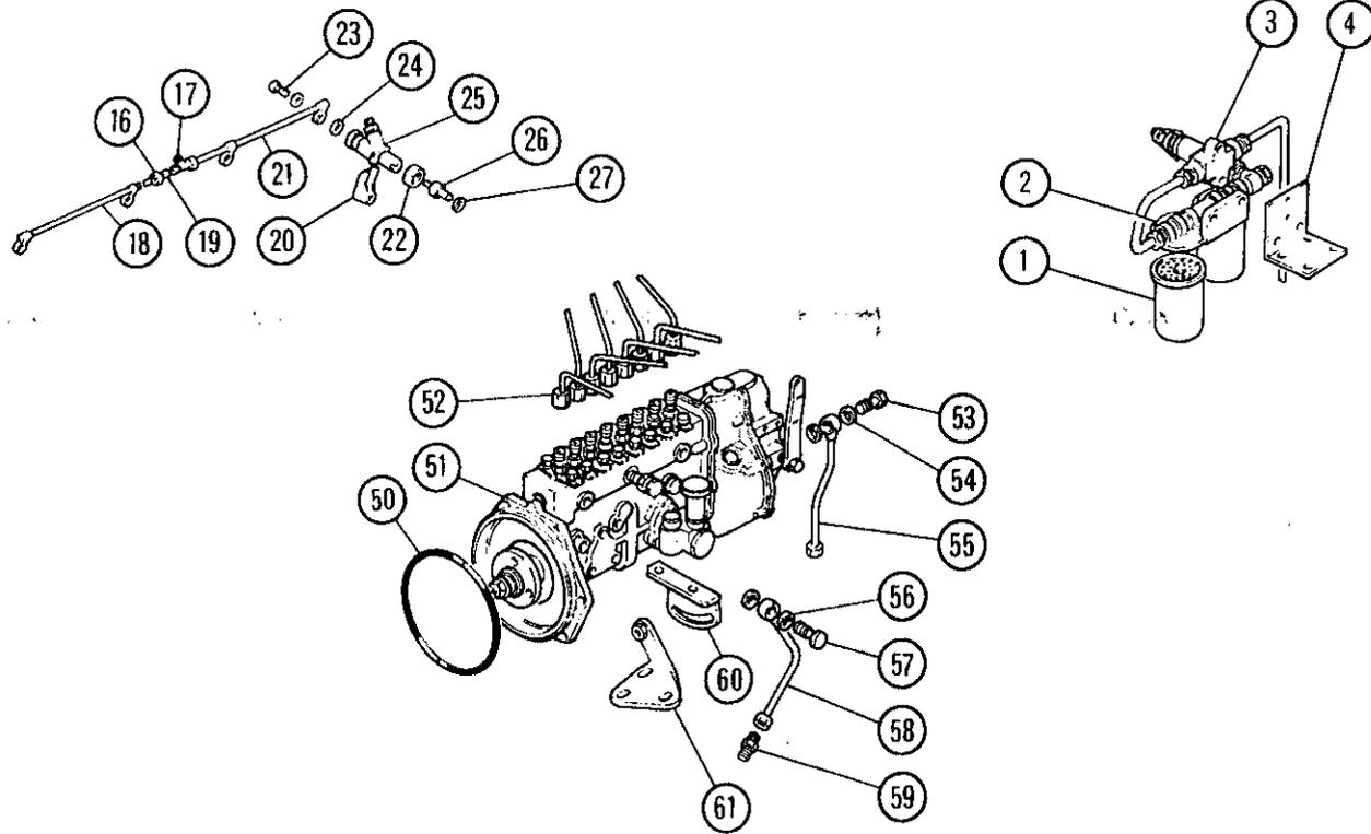
Fig. 31 Fuel system components (in line pump)
