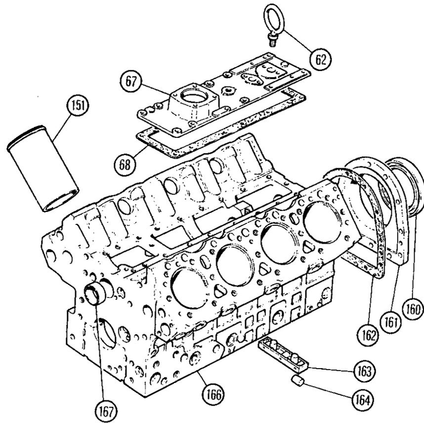
Fig. 27 Cylinder block assembly
