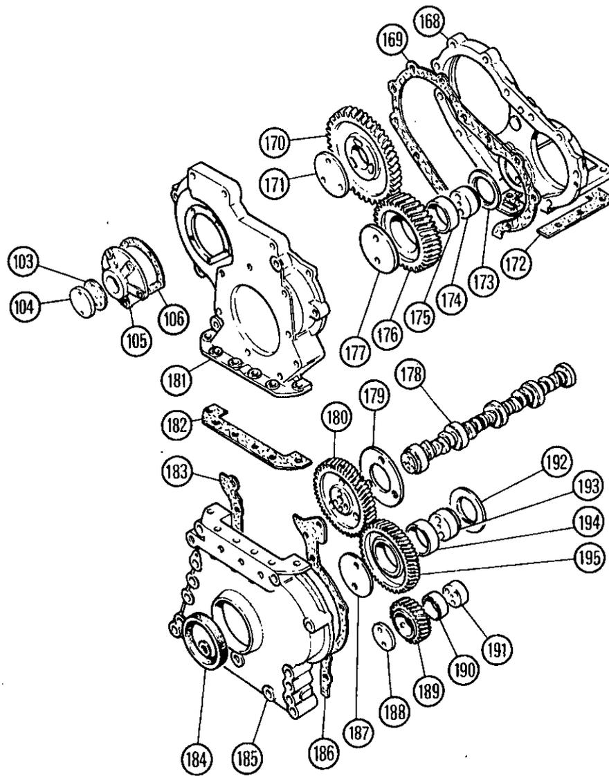
Fig. 28 Timing case and drive arrangement
