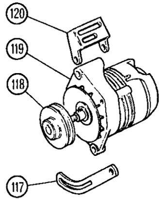
**Fig. 32** Alternator and brackets
