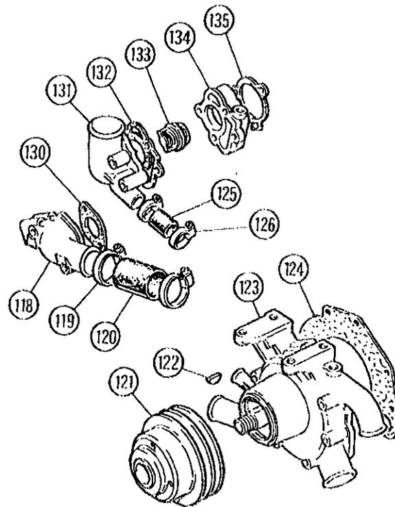
**Fig. 35** Cooling system components
