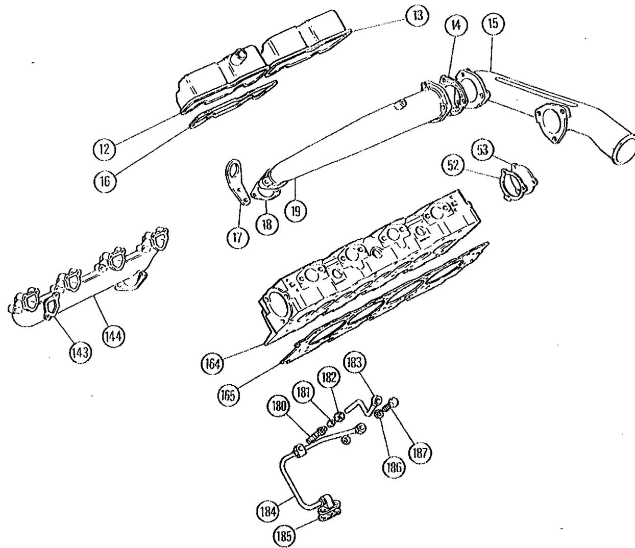
Fig. 29 Cylinder head arrangement
