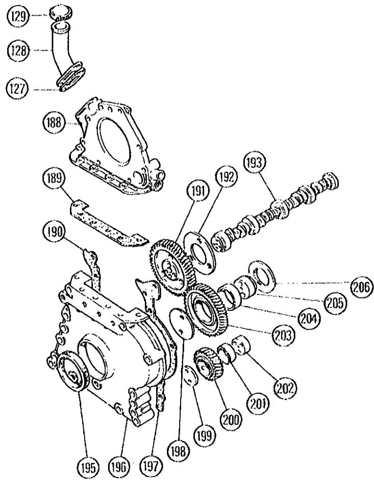
**Fig. 33** Timing case and drive arrangement
