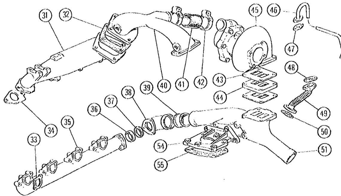
Fig. 39 Turbocharger system
