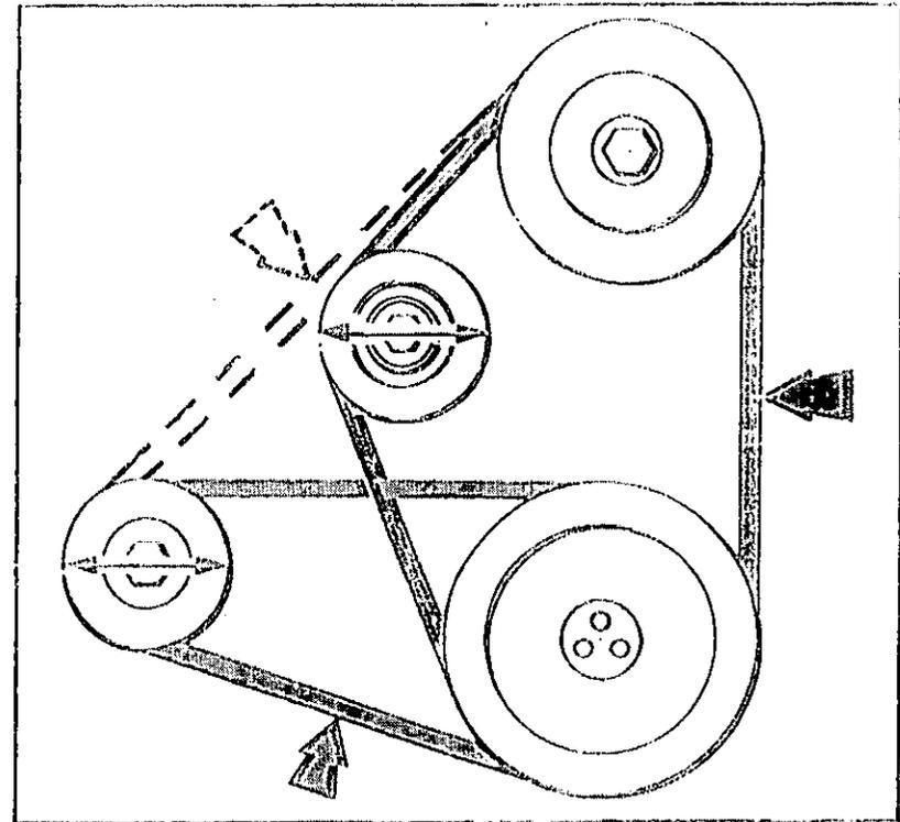
Fig. 13 Drive belt tension adjustment
