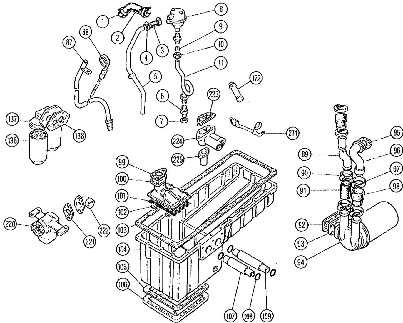
Fig. 34 Lubrication system components
