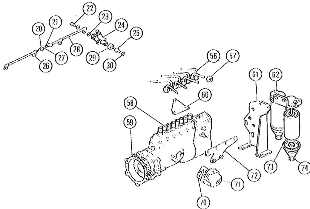
Fig. 36 Fuel system components (in line pump)
