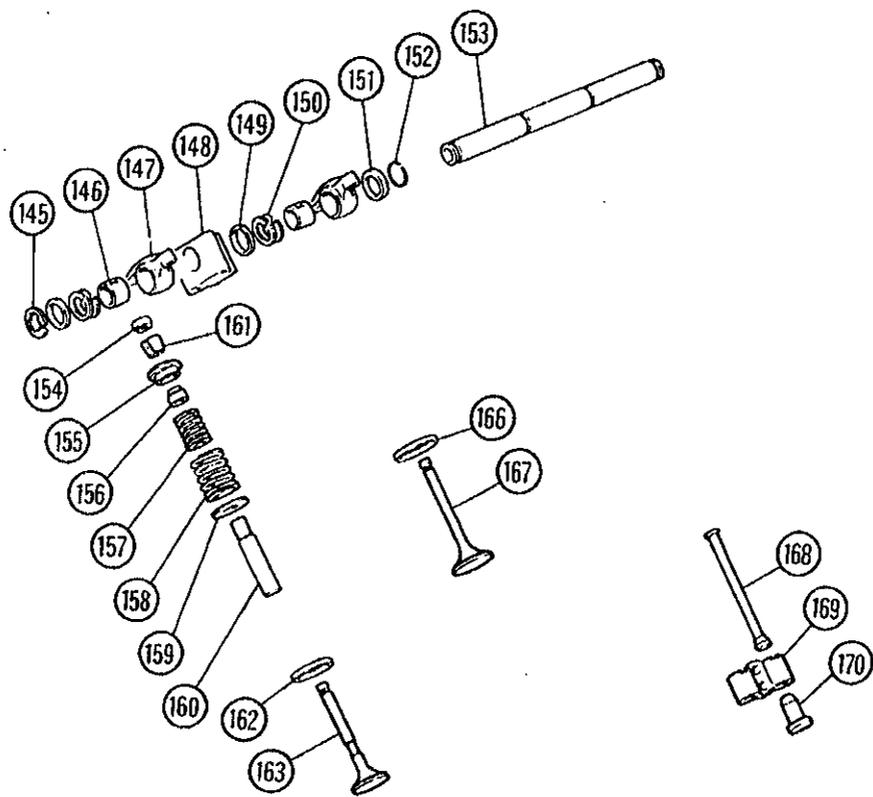
Fig. 30 Valves and rocker assembly
