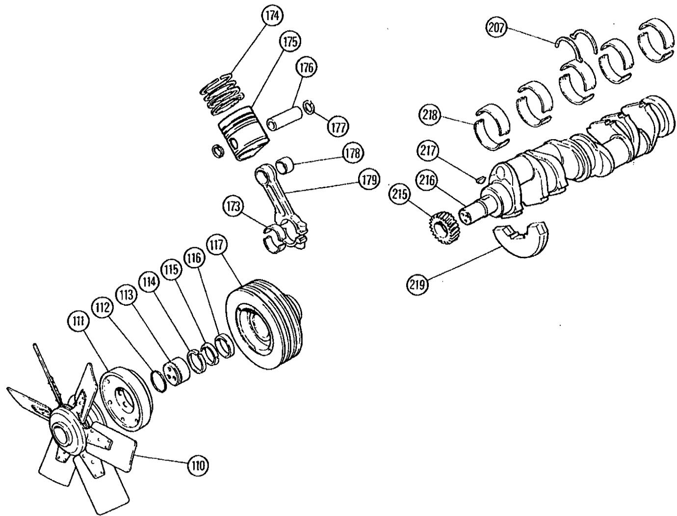
**Fig. 31** Crankshaft and piston assemblies
