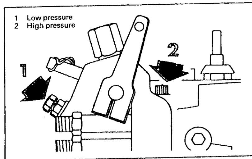
**Fig. 23** CAV rotary fuel injection pump vent points
