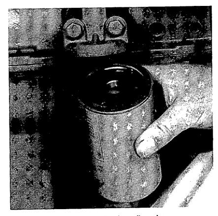
Fig. 8 To renew the lubricating oil canister
