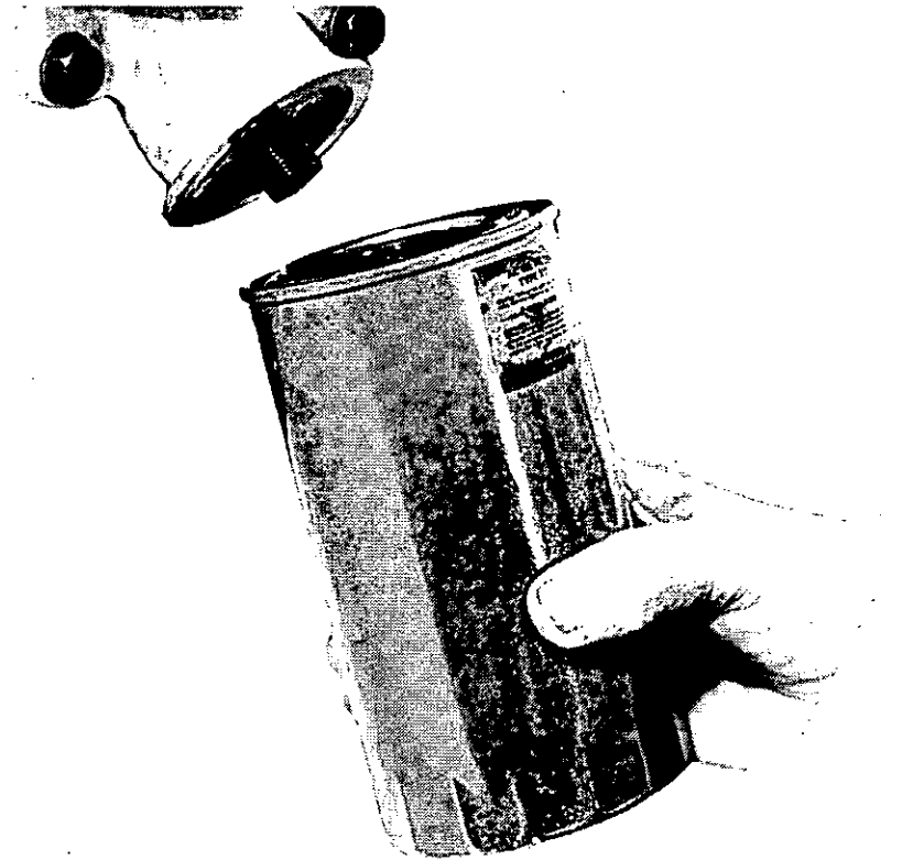
Fig. 9 To renew lubricating oil filter canister
